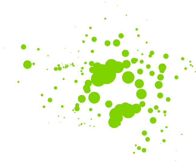
Figure 1.3: One of the images from “Green-graphs & IRIS” presenting multi-operator base station deployment around the Cork city area, with cell radius denoting the local value of a specific summary characteristic and the colour denoting frequency used by the base stations.
