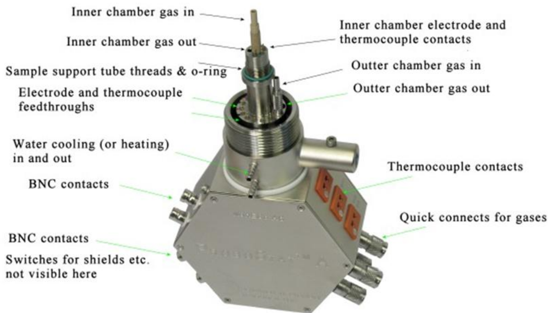
Figure 3.3. Probostat™ base unit with feed throughs.
