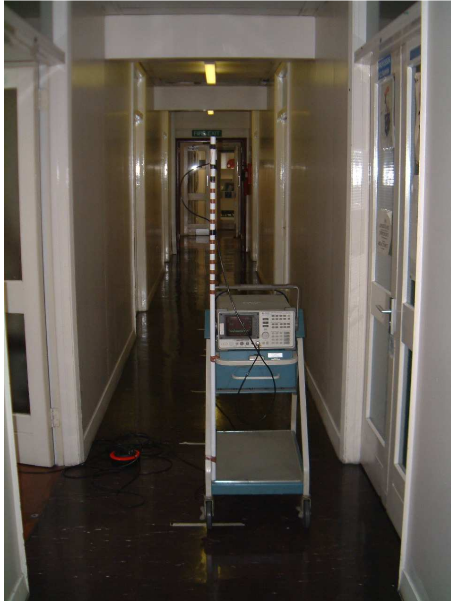
Figure 5-9: A trolley with a half-wave dipole antenna set up to measure incoming signals from another antenna.
