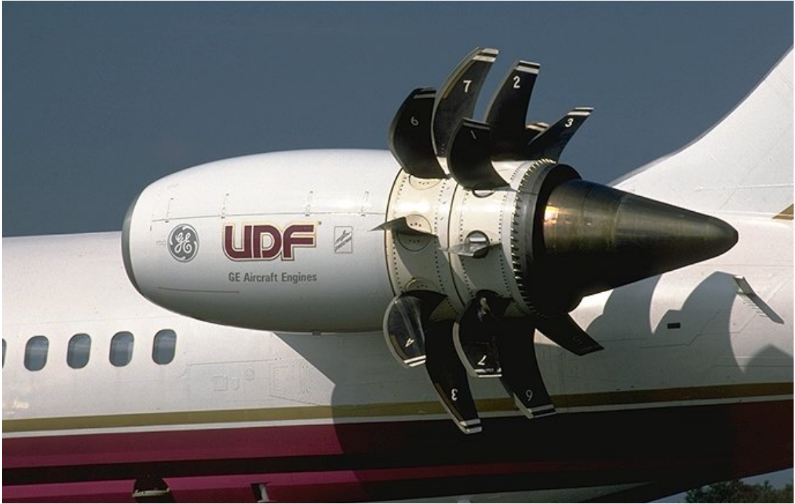
Figure 1: GE Unducted Fan mounted on an MD-80[27].
