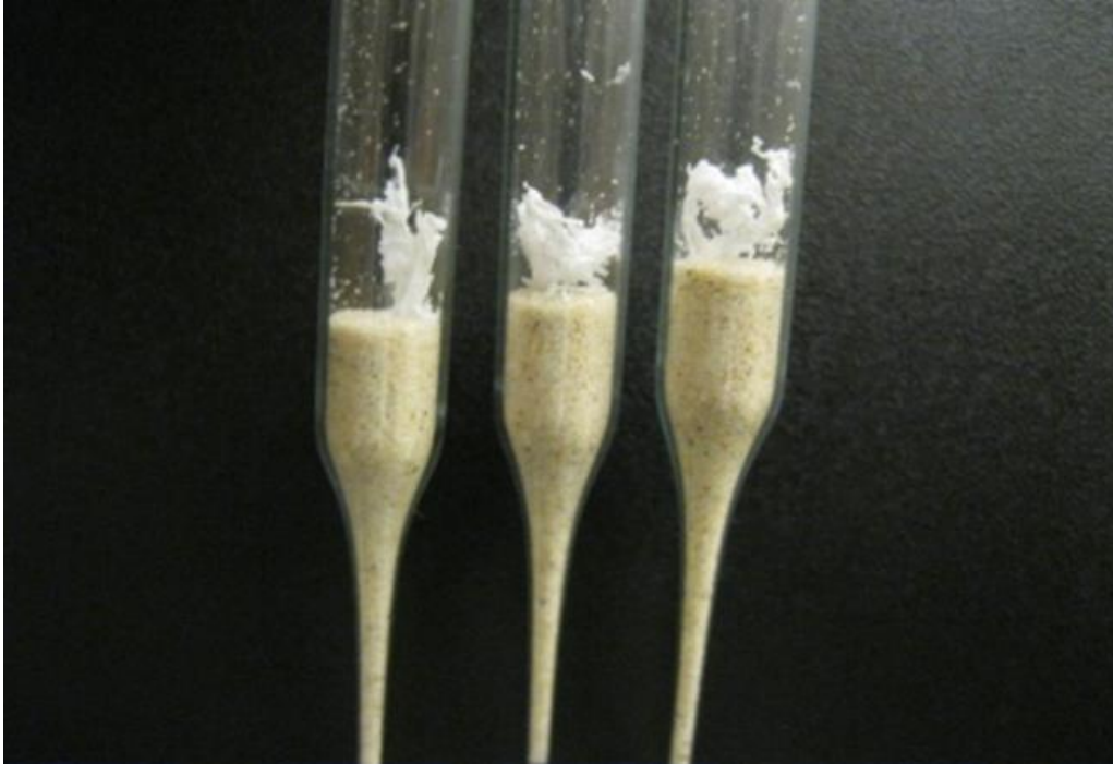
Figure 46 Glass pipets with control sand and mucilage nanofibers [8]
