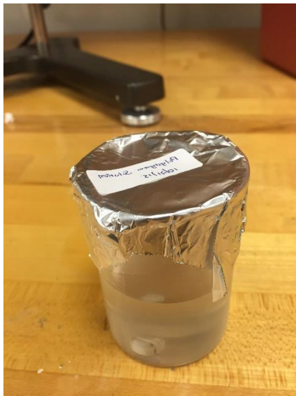
Figure 8 Polystyrene solution with D-limonene at 20% by weight ratio
