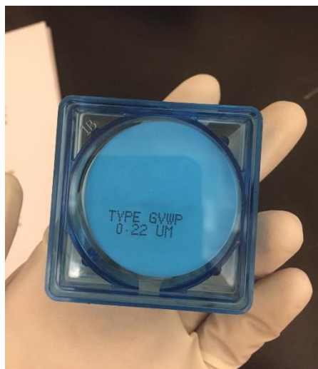
Figure 45 GVWP durapore membrane with pore size 0.22 \mu\text{m}
