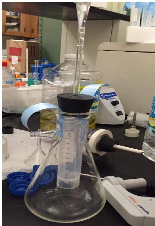
Figure 47 Filtration system setup for testing arsenic contaminated water
