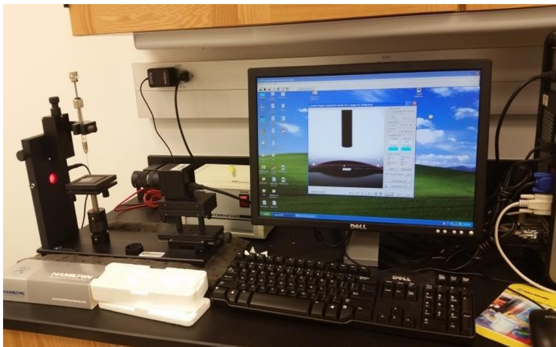
Figure 34 Contact angle measurement (CAM) system
