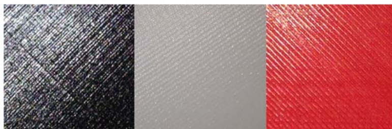
Figure 2.4 Surfaces of FDM parts
