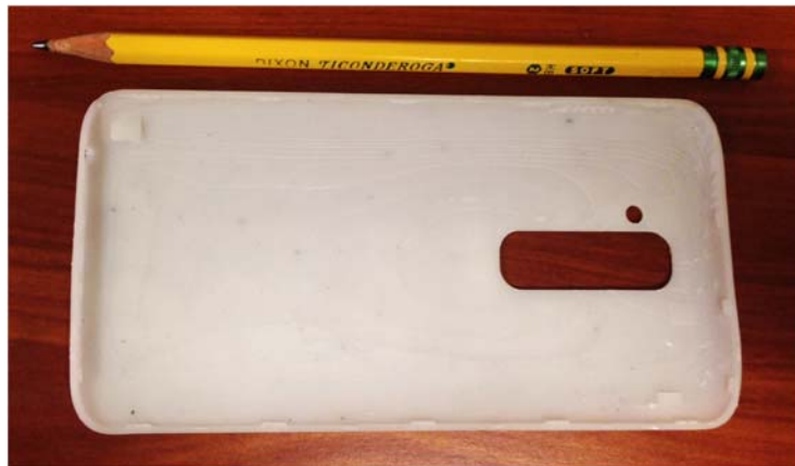
Figure 2.10 Nanotool phone cover with smooth surface finish printed via Stereolithography
