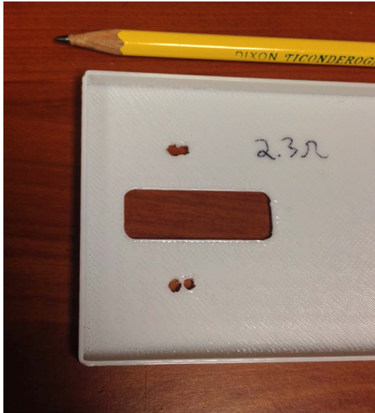
Figure 2.2 Polycarbonate phone cover with surface valleys printed via FDM
