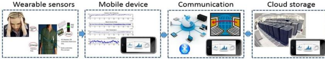
Figure 4.1: Hardware architecture of a context-aware mobile system.
