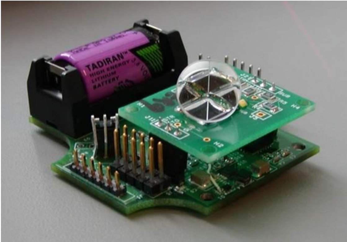
Figure 6-1: Assembled transmitter unit with temperature, humidity, and 2-axis magnetic sensors; microcontroller; infrared remote control receiver; field configuration jumpers; and a battery. The unit was housed in an IP-67 enclosure with transparent acrylic walls.
