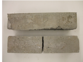
Figure 5.9: Comparison of PCM and rubber specimens under flexural testing.
