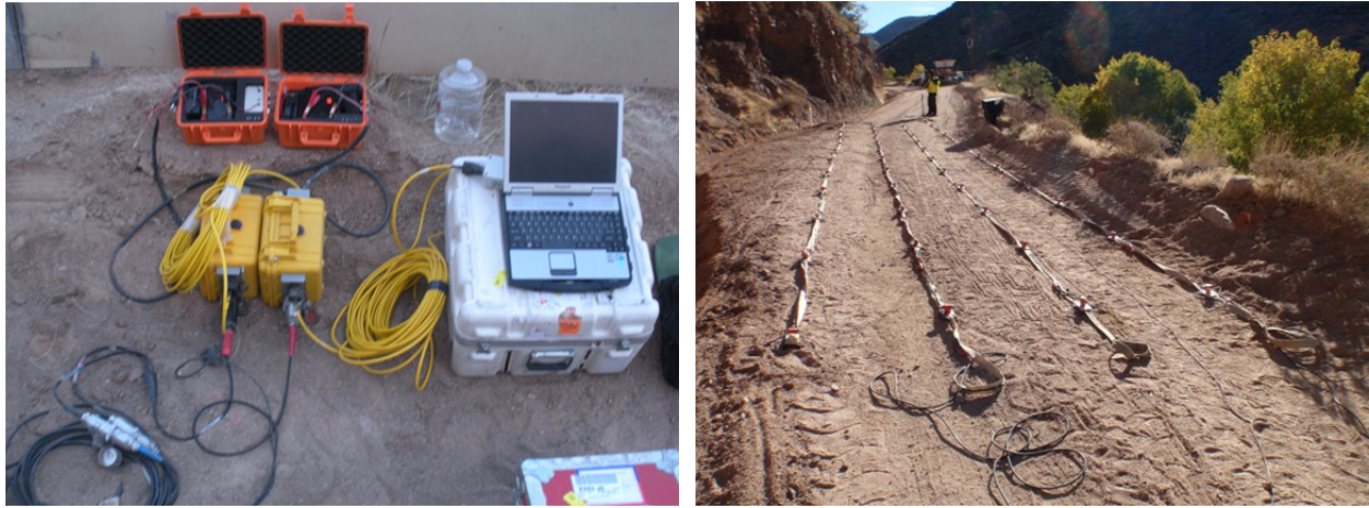
Figure 5.4. (L) Laptop, seismograph, and battery setup; and (R) geophones deployed on landstreamers at Apache Trail.
