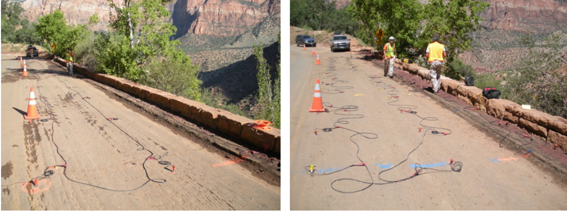
Figure 4.3. Layouts of the (L) 10-ft (3-m) geophone spacing for grid #1 and (R) 5-ft (1.5-m) geophone spacing for grid #1 at Zion N.P. during pre-grouting seismic data collection.
