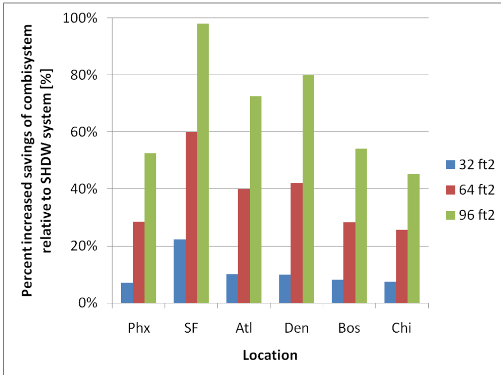
Figure 5.41: Impact of climate on the relative increase in savings from the combisystem as compared to a SHDW for a low load house (20 gallon draw/BA 50% House)
