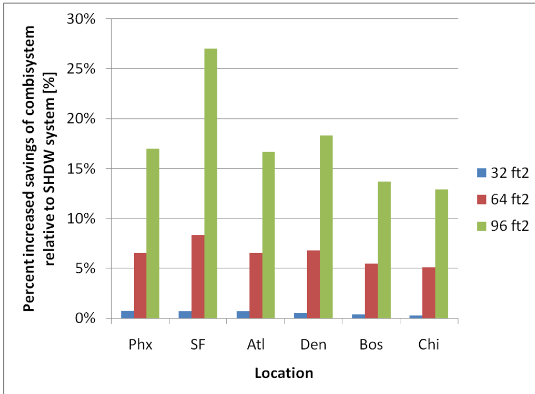
Figure 5.34: Impact of climate on the relative savings increase of the combisystem relative to the SHW for three collector area sizes (Benchmark House/60 gallon draw)
