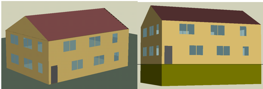
Figure 4.17. The renderings for the homes that were modeled. The building on the left is slab-on-grade construction, while the home on the right has a basement and was used for the colder climates (Denver, Boston, and Chicago).
