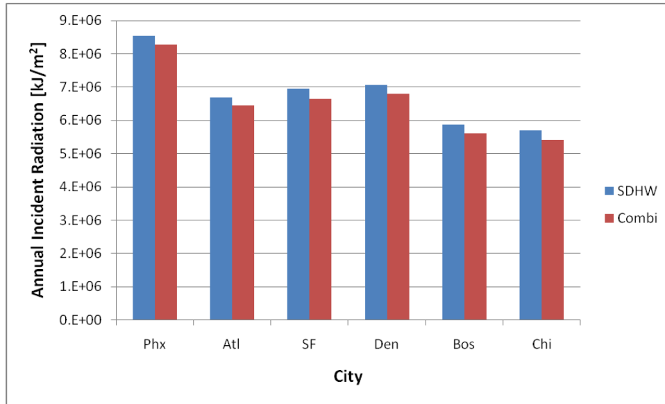
Figure 5.36: Annual specific incident radiation levels on collectors for SWH and Combi system in all the
