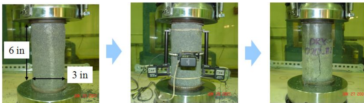
Fig.8.1 Set-up and procedure of compression test
