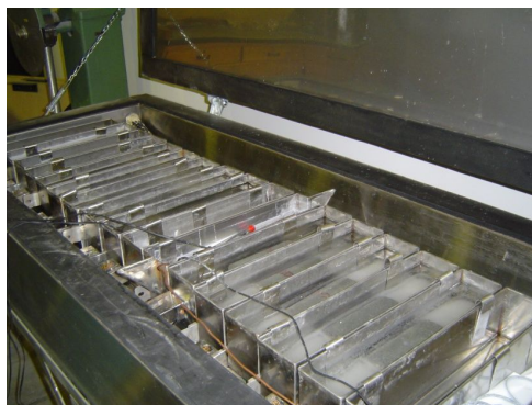
(b) Frozen specimen after 30cycles
