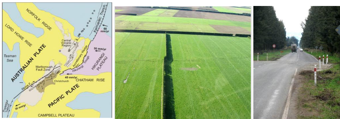
Figure 4-1.a. Fault zone in New Zealand. 1b. Greendale fault 1c. Road offset due to fault (Jongens et al., and Begg, 2010)
