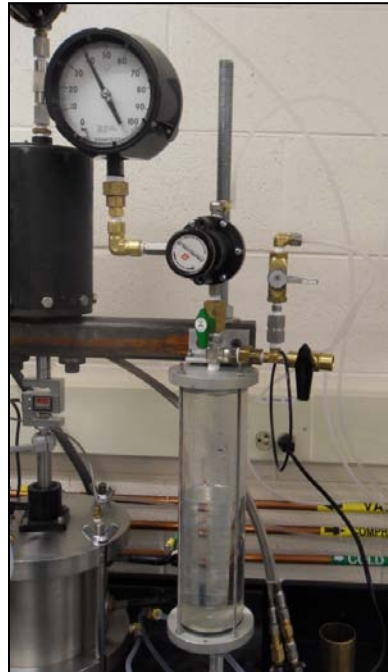
Fig. 4.9: Closed, glass pressure reservoir
