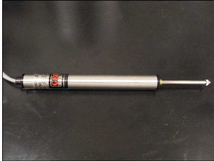
Fig. 4.8: LVDT model E-312 used to measure the axial deformations
