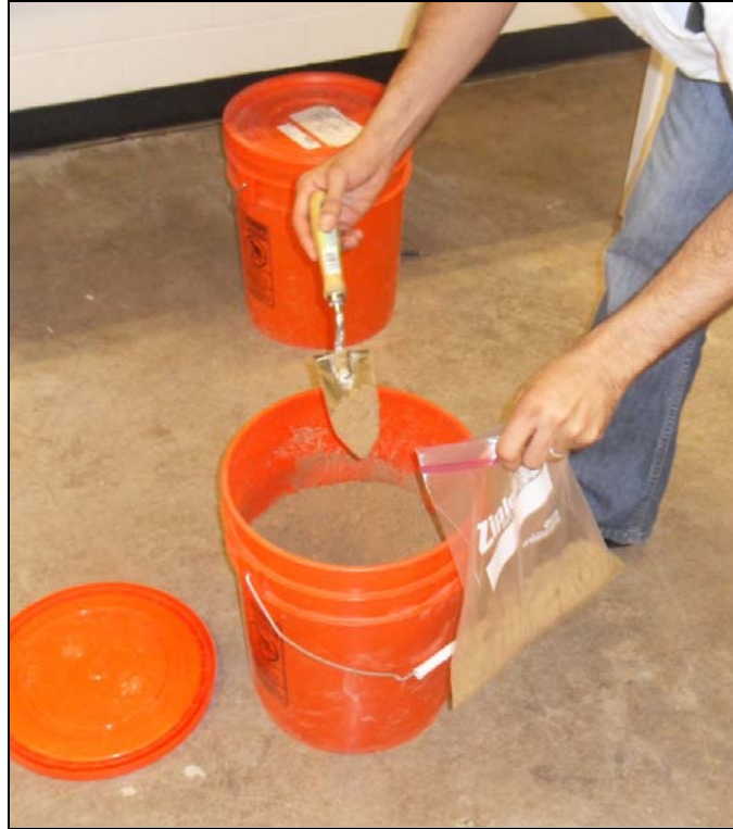
Fig. 5.1: Moisture conditioning of soil
