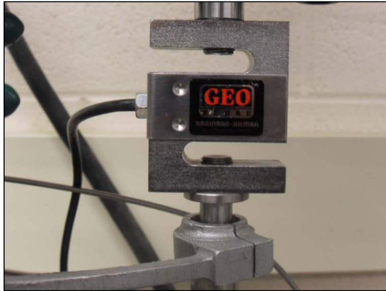
Fig. 4.7: Load cell used to measure the axial load applied to the specimen
