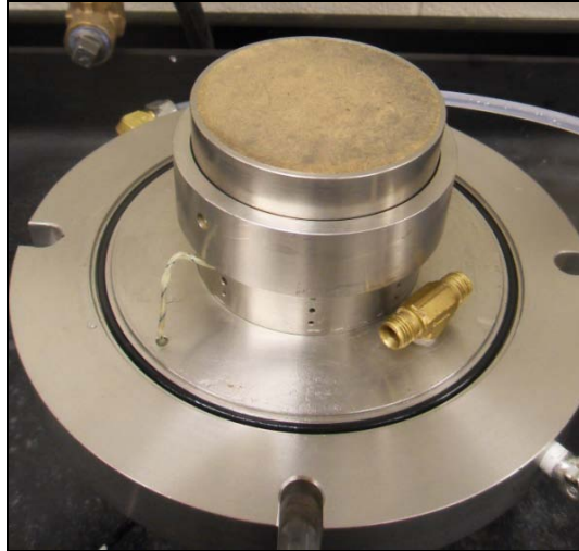
Fig. 5.7: The consolidation ring containing the specimen inside the pressure cell
