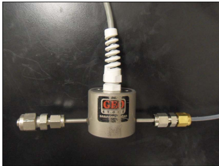
Fig. 4.11: Pressure Transducer model E-124 used to measure pore water pressure
