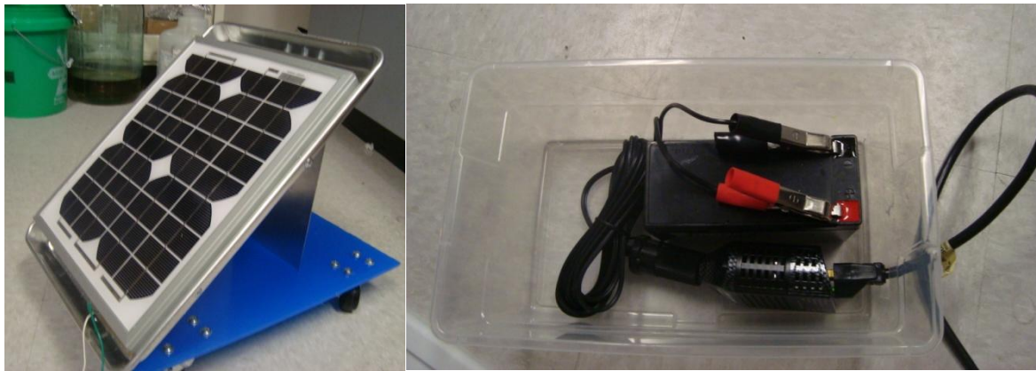
Figure 13. Solar panel and mounting system (left), and balance of systems (right) of design 1.
