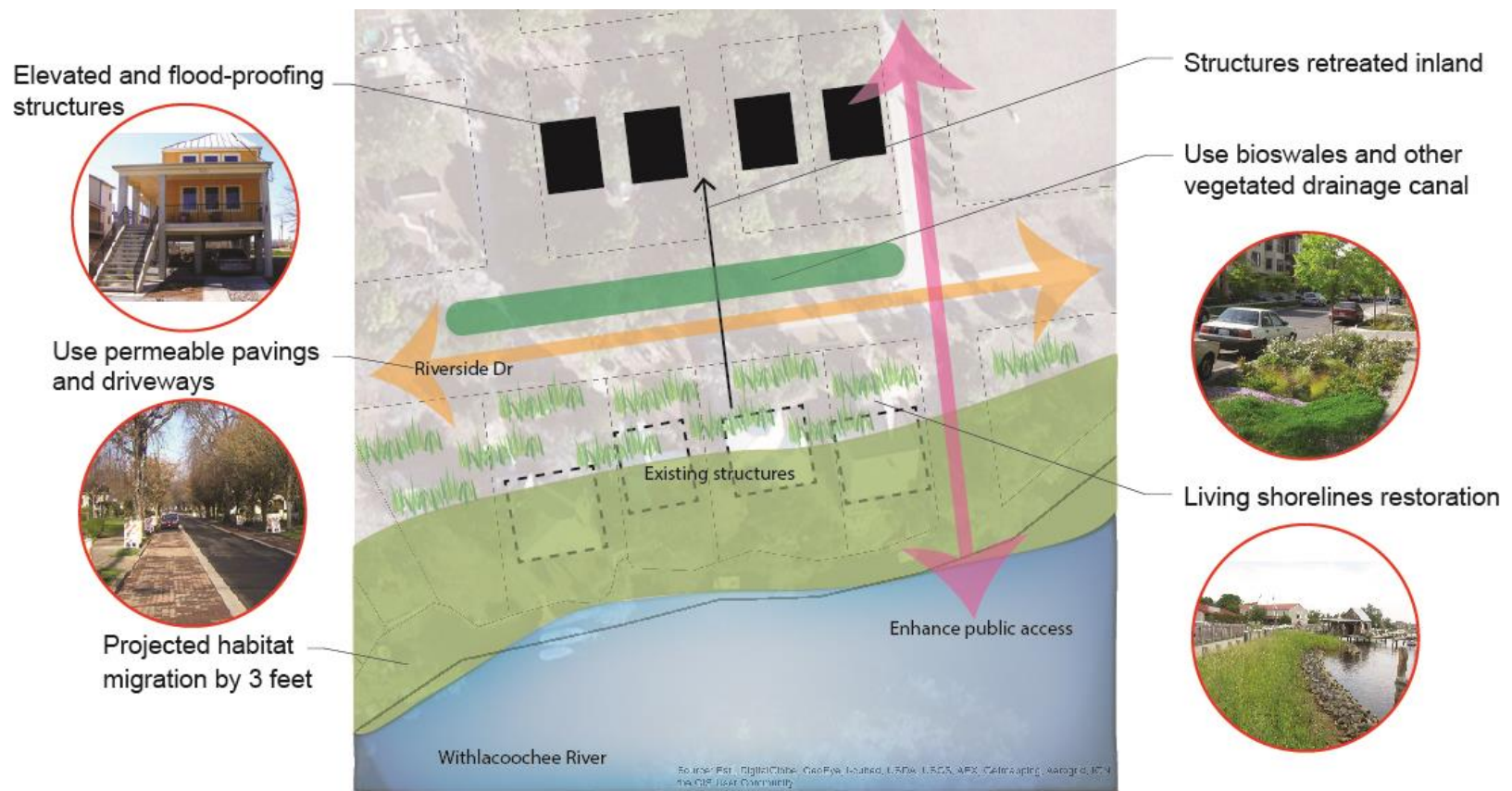
Figure 5-11. Adaptation Strategies Scenario I—waterfront design. Source of images: FloodProBE, n.d.; City of Berkeley Department of Public Works, n.d.; Eye On Annapolis, 2011.
