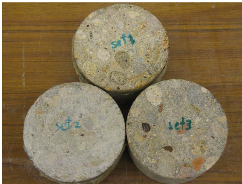
Fig. F.1 Concrete specimens for Rapid Chloride Permeability Test
