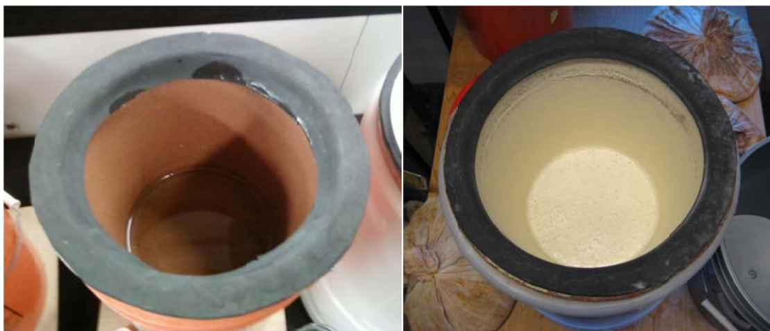
Figure 5-20: CWF before 500 NTU and after 500 NTU loading
