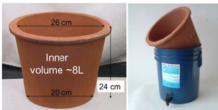
Figure 1-1 Typical CPF produced by Potters for Peace Factory in Nicaragua (PFP 2006)
