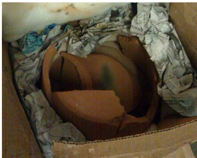
Figure 6-52 Broken ceramic pot filter after being shipped from Nicaragua
