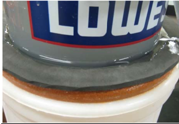
Figure 6-51 Water pooling between the top bucket and the gasket
