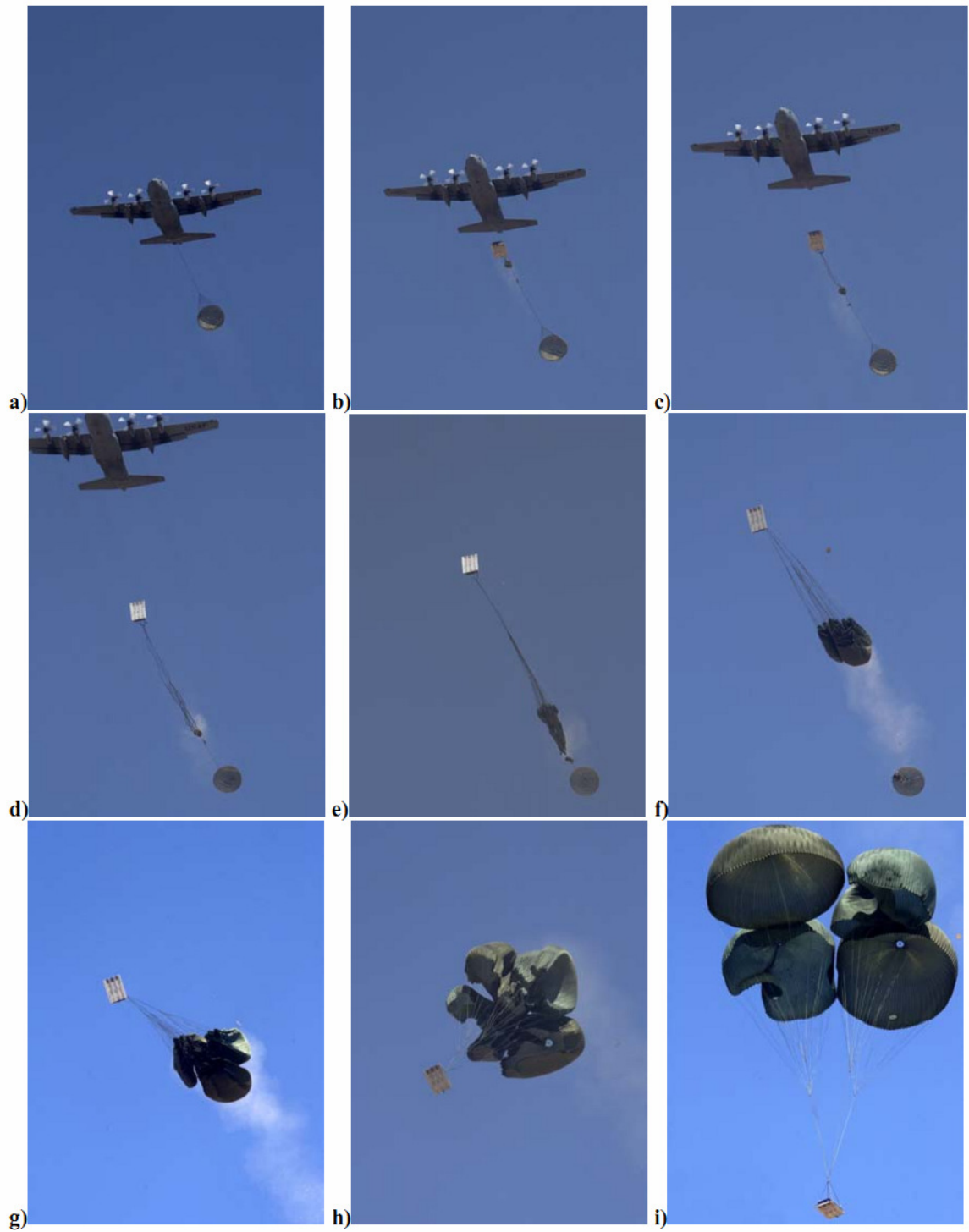
Figure 1.2: Opening Sequence for Payload Delivery with Multiple Round Parachutes [6]
