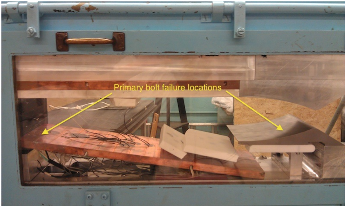
Figure 3.11: Failure of lower testing surfaces. Arrows indicate locations of bolt failures.
