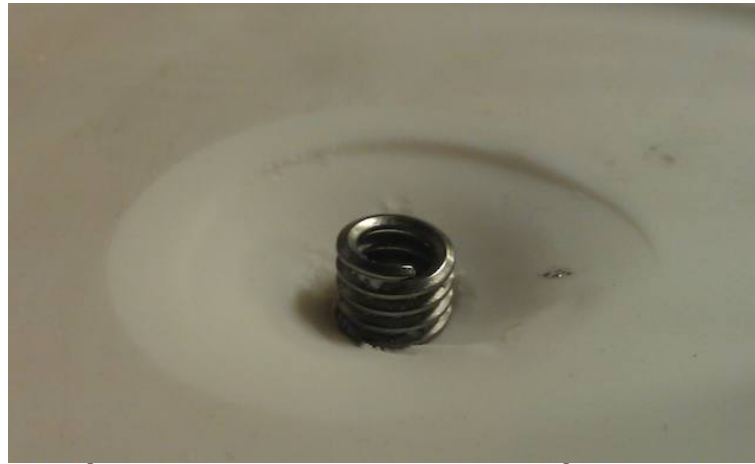
Figure 3.17: Heli-Coil ® insert and failure of surrounding MACOR ® surface.
