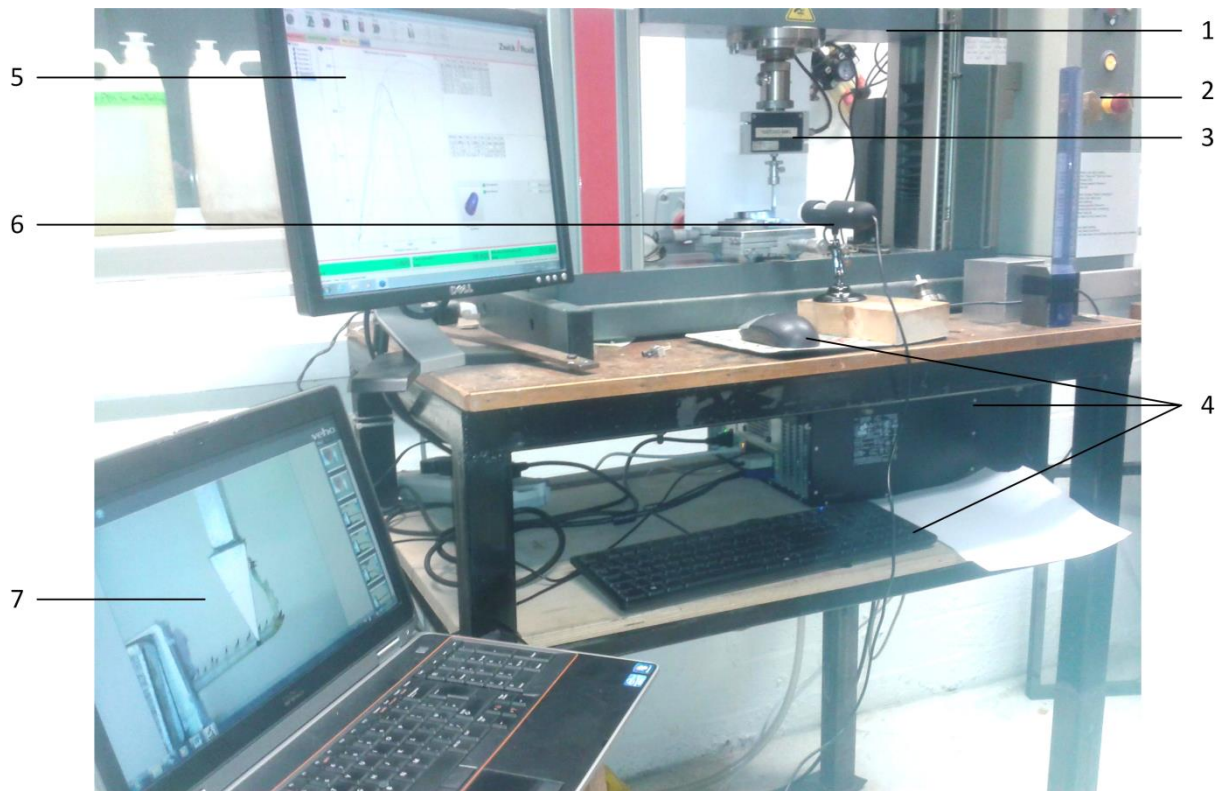
Figure 2.3: the experimental setup. 1: the Zwick tensile / compression testing machine. 2: the manual control panel. 3: the 5 N load cell. 4: the computer equipment for controlling the Zwick machine. 5: the graphical user interface of the TextExpert software displaying force-displacement curves. 6: USB microscope for monitoring / photographing samples during tests. 7: the display and user interface of the USB microscope.
