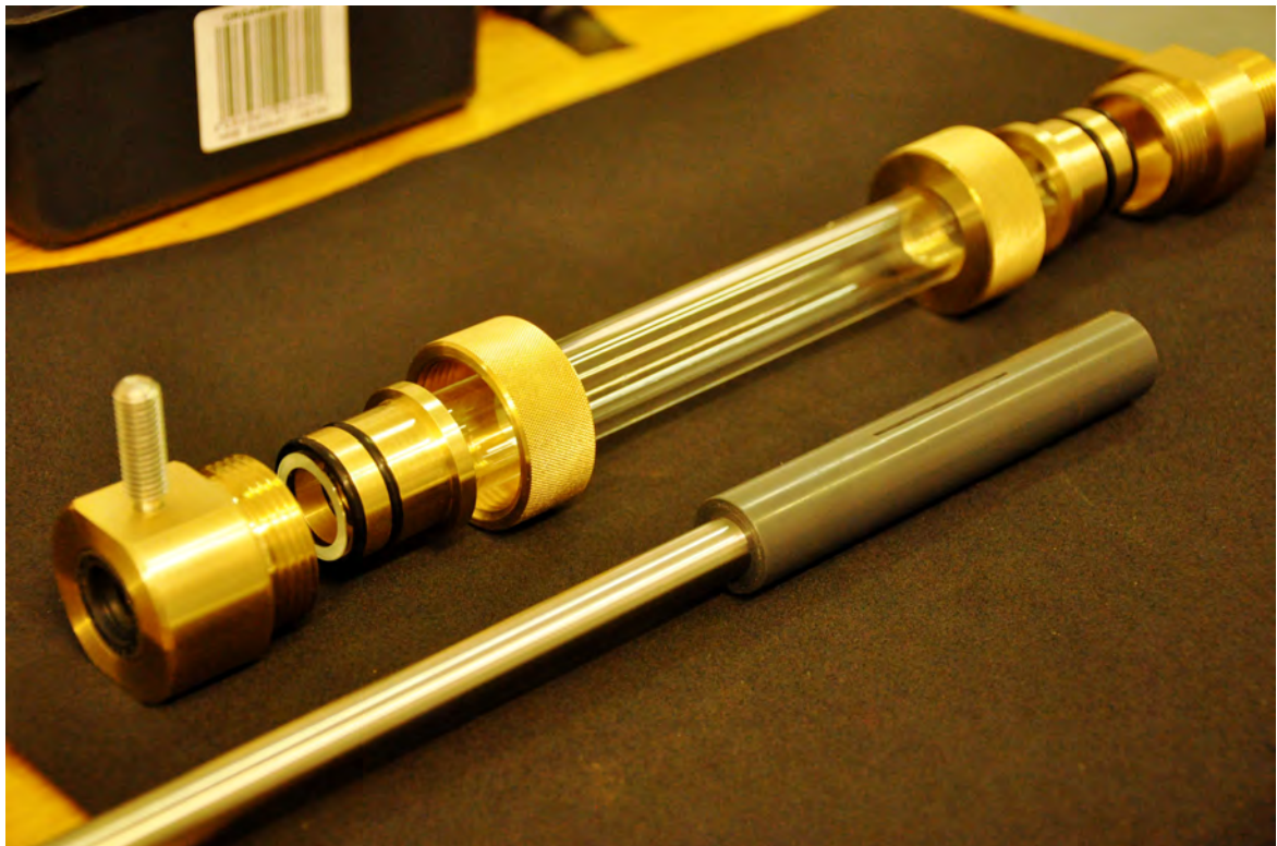
Figure 3.21: Cylinder with embedded synthetic jet, and test section sting arm
