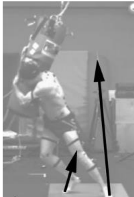
Figure 17. A staged shoulder tackle on an instrumented tackle bag in a motion analysis laboratory [173]. Both the tackler and tackle bag were instrumented with retro-reflective markers. The black arrows illustrate the force plate measures.
