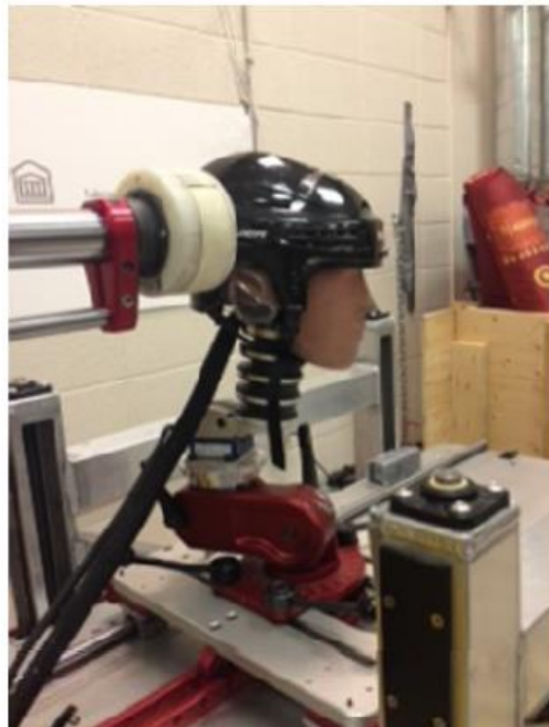
Figure 14. Laboratory reconstruction of a concussion event with a linear impactor and ATD head and neck model [148].
