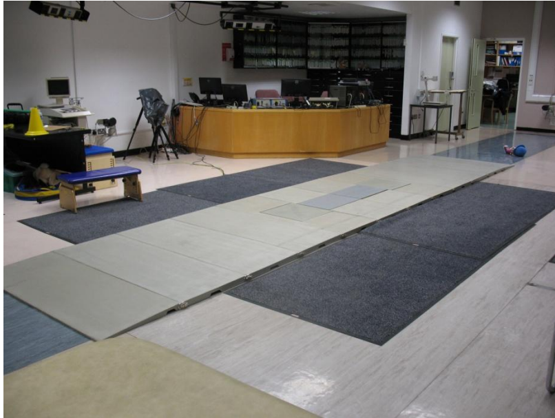
Figure 5.11: Fibreglass walkway configuration to incorporate additional AMTI force platforms in the current CRC gait laboratory setup.
