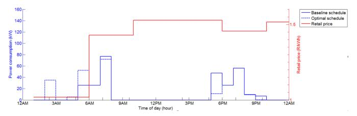
Figure 5.5: Optimal and baseline schedule as well as retail price over a 24-hour cycle when the battery is active
