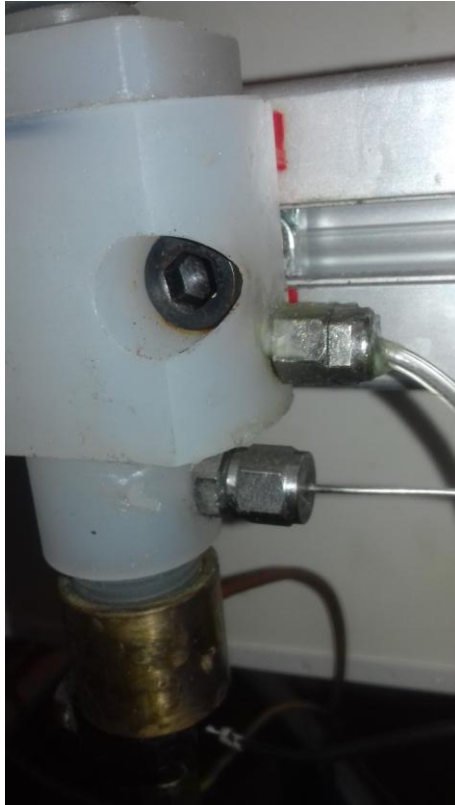
Figure 4-7. Type-T thermocouple with sealing gland
