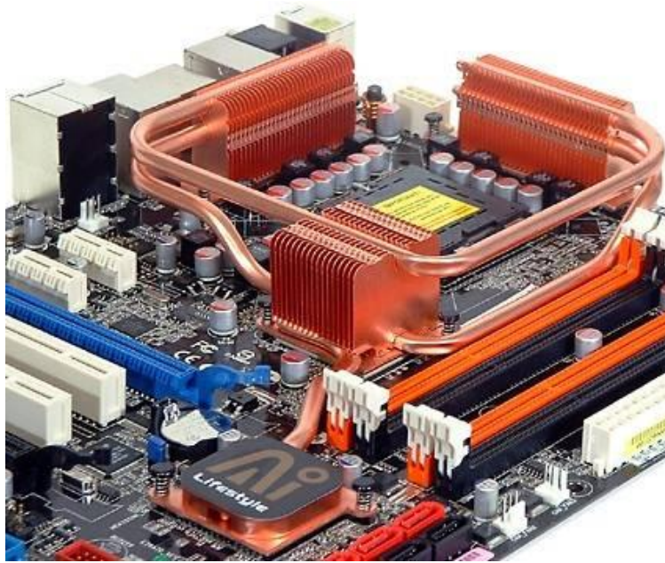
Figure 1-3. Heat pipes built on P35 Express motherboards [11]
