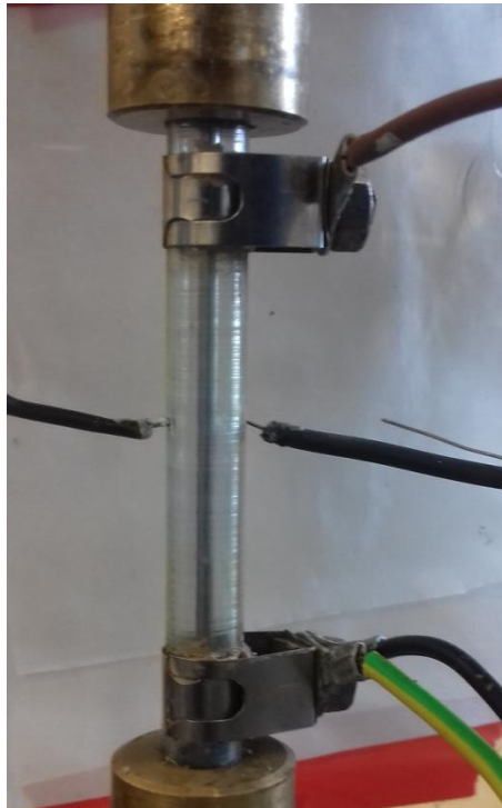
Figure 4-8. Test section, conductive clamps and thermocouples position
