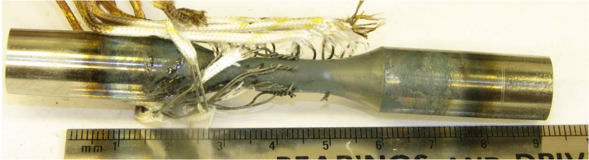
Figure 3-4: Induction Coil Verification: 4 Thermocouples Welded Circumferentially Around Center of Gage Section
