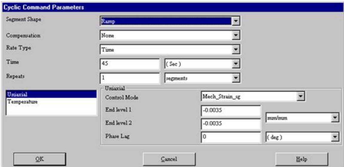
Figure A-6 OP TMF “Initial TMF Cycle (0-.25)”- Go To T_{max} and \epsilon_{min}
