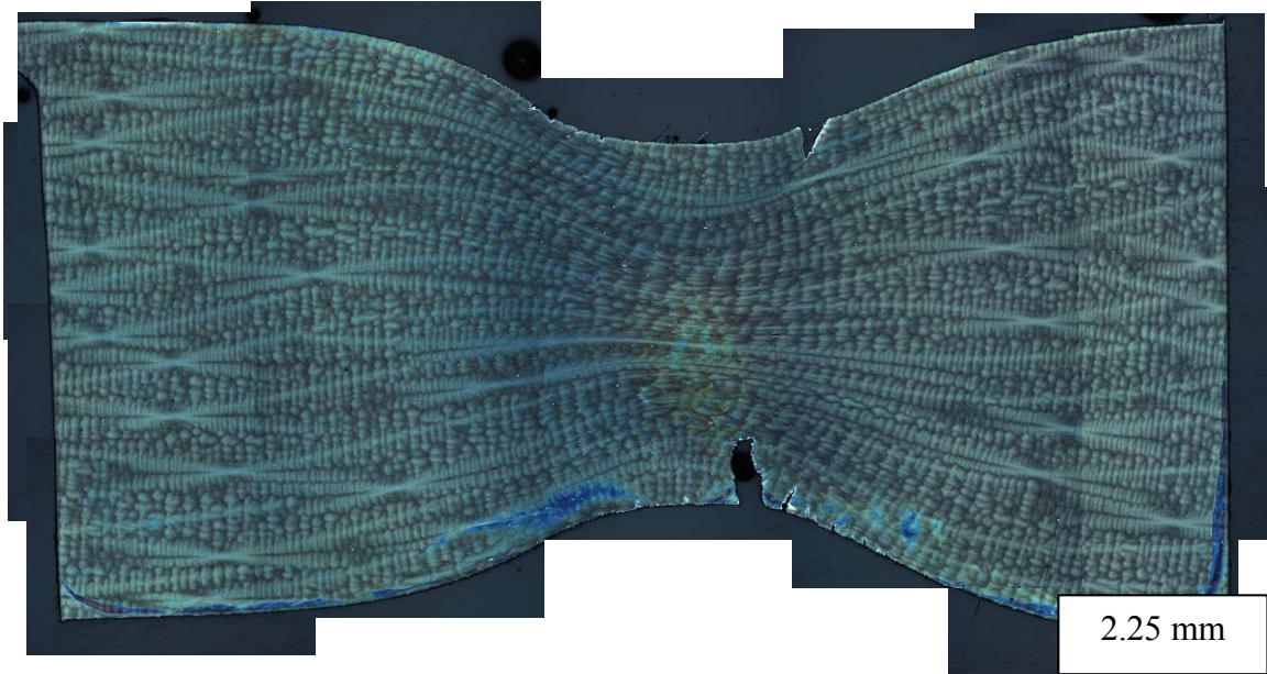
Figure 3-41 Specimen Cross-Section: <001> Orientation, 1.3% OP TMF 5 min High Temperature Hold- loading direction horizontal
