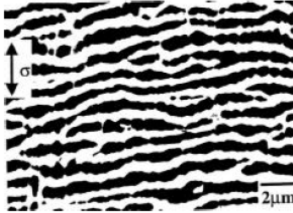
Figure 2-29 Micrograph of Rafting in a Single Crystal Superalloy [19]
