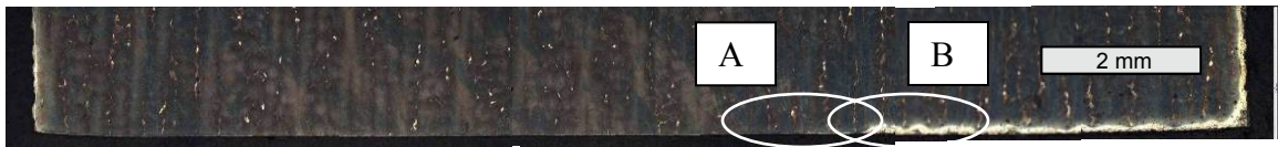
Figure 4-10 Top: Specimen Tested at 1050°C for 300 hours. Bottom: Cross Section A-A
