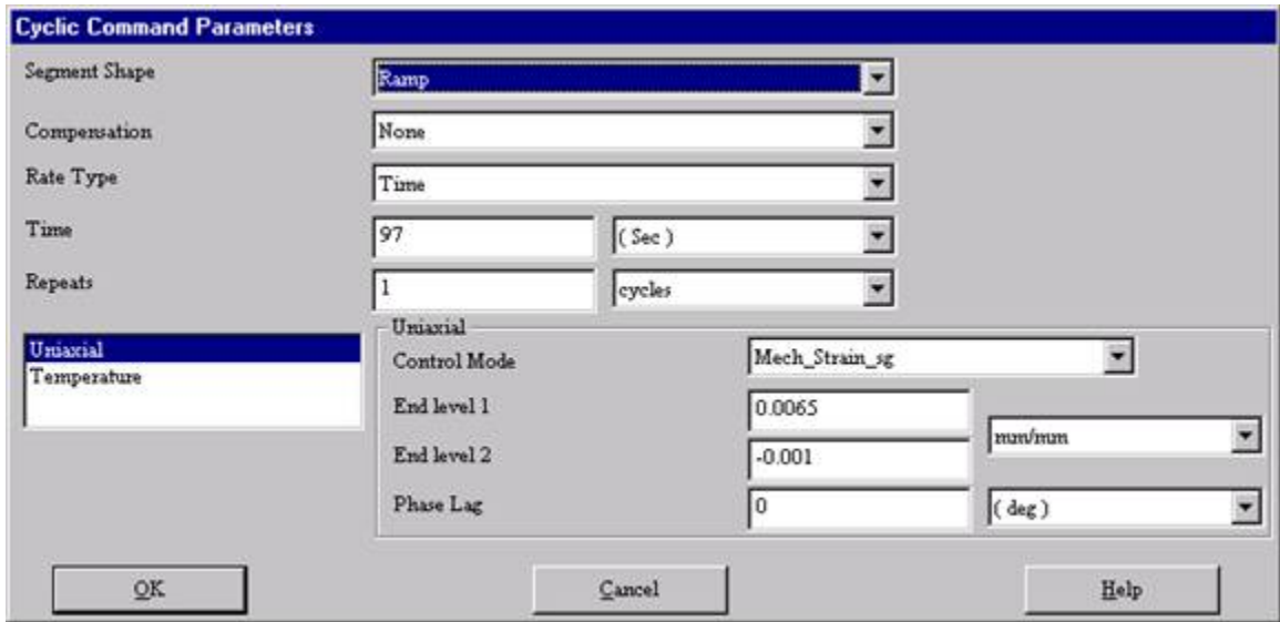
Figure A-14 OP BiF Control Loop “high temp load”- Tensile Half Cycle
