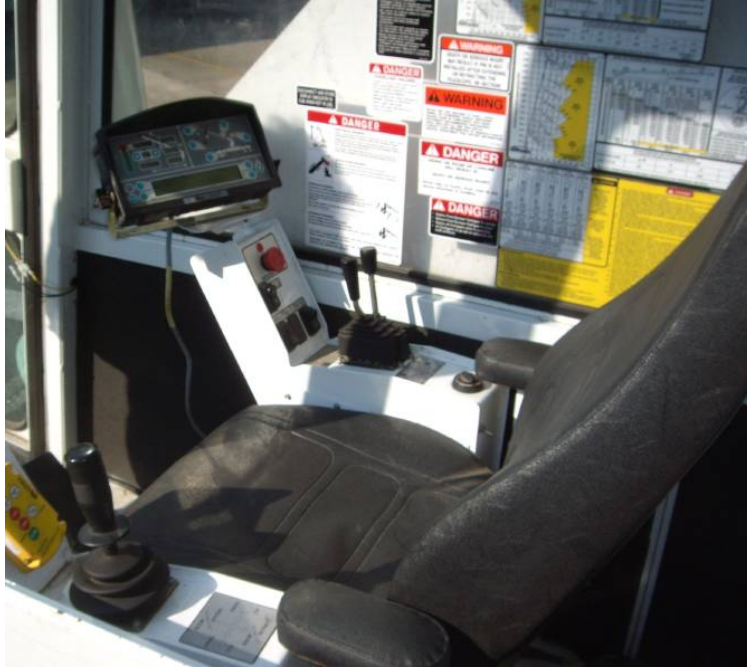
Figure 8: Excessive Warning Labels in the Cab
