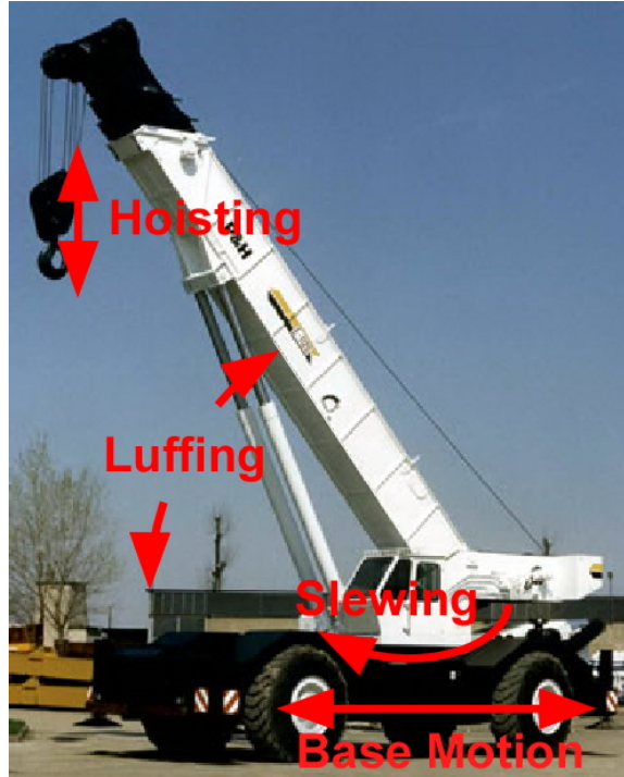
Figure 2: Mobile Boom Crane and Common Crane Motions [36]
