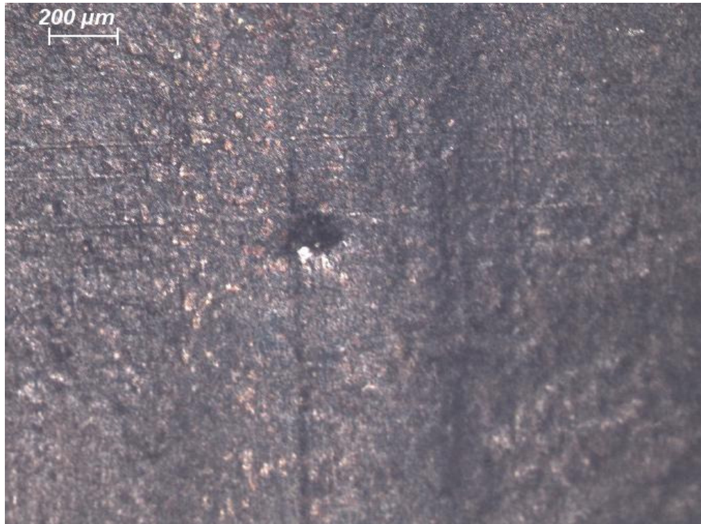
Figure 5.30: Damaged Part of the Seal.
