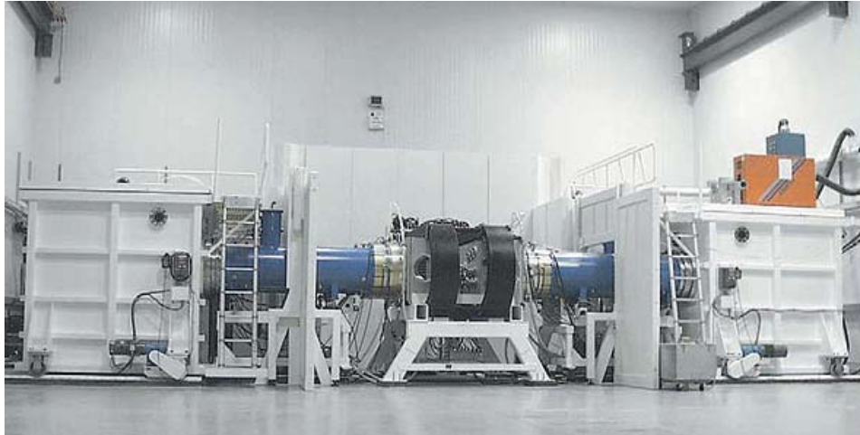
Figure 1-2 Electra at the NRL (laser cell open and recirculator detached, Sethian, et al , 2001)
