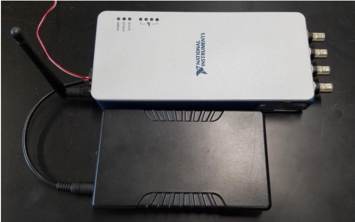
Figure 5.1: NI cDAQ-9191 Wi-Fi chassis and lithium ion battery pack.
