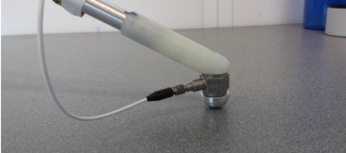
Figure 5.3: White cane with force gauge mounted to its tip.
