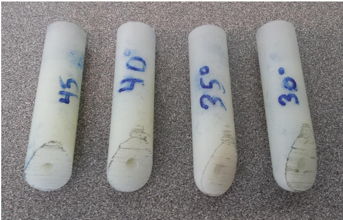
Figure 5.2: Modified cane pencil tips, used to mount force gauge to cane tip.
