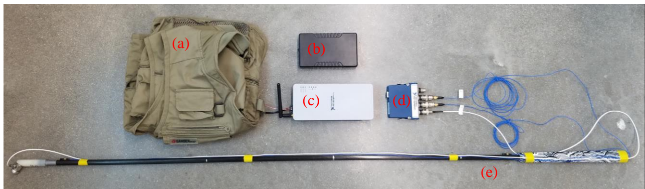
Figure 5.6: (a) Fishing vest, (b) battery pack, (c) Wi-Fi chassis, (d) data acquisition module, and (e) instrumented cane.
