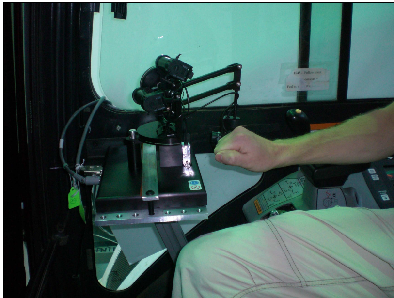
Fig. 23 Phantom Mounted in the Cab. The Phantom was mounted so that operators could use the stock excavator armrest to support their forearms.
