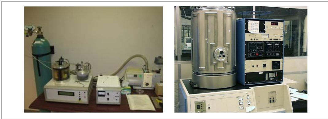
Figure 2.6: (Left) Gold Sputtering Unit (Right) CVC E-Beam Evaporator (courtesy of Georgia Institute of Technology)
