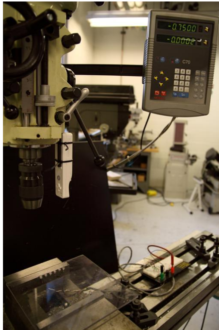
Figure 21: Wii Remote™ calibration test setup
