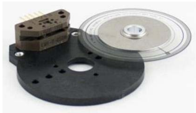
Figure 18. Optical encoder components (U.S. Digital Inc.)
