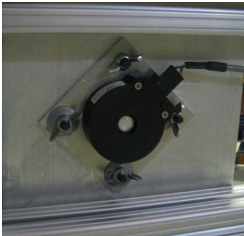
Figure 20. Encoder mounted to bottom of iMachine frame
