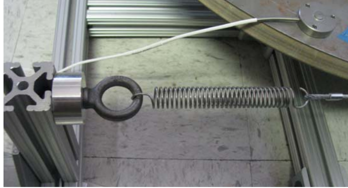
Figure 15. iMachine extension spring in static equilibrium
