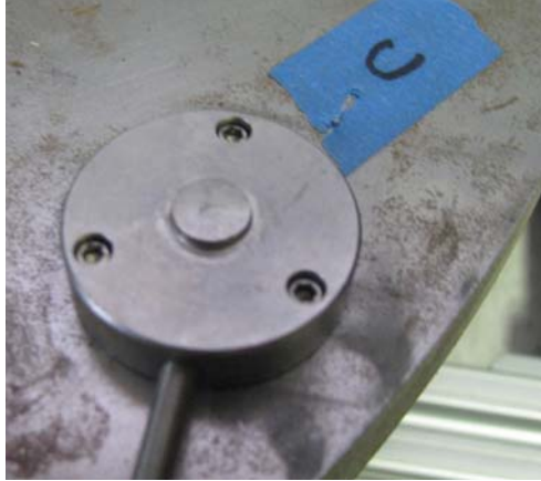
Figure 17. Load cell mounted to iMachine disk
