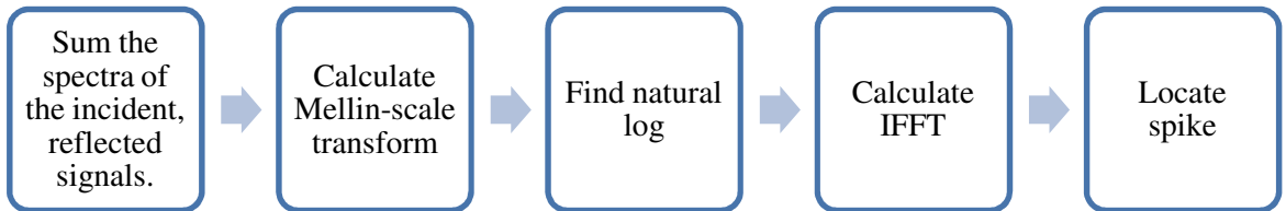
Figure 9 – Doppler method for velocity detection
