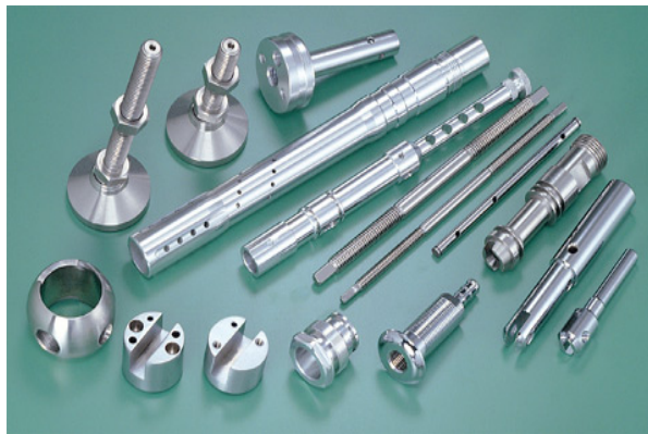
Figure 1.1: Cylindrical components produced by the centerless grinding operation
