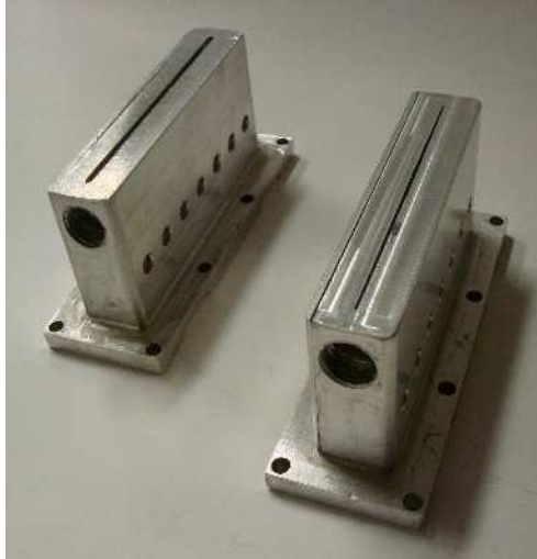
Figure 2.3: Photograph of inner cartridges with 2 mm (left) and 0.5 mm (right) wide slots; inlet port is visible for both cartridges
