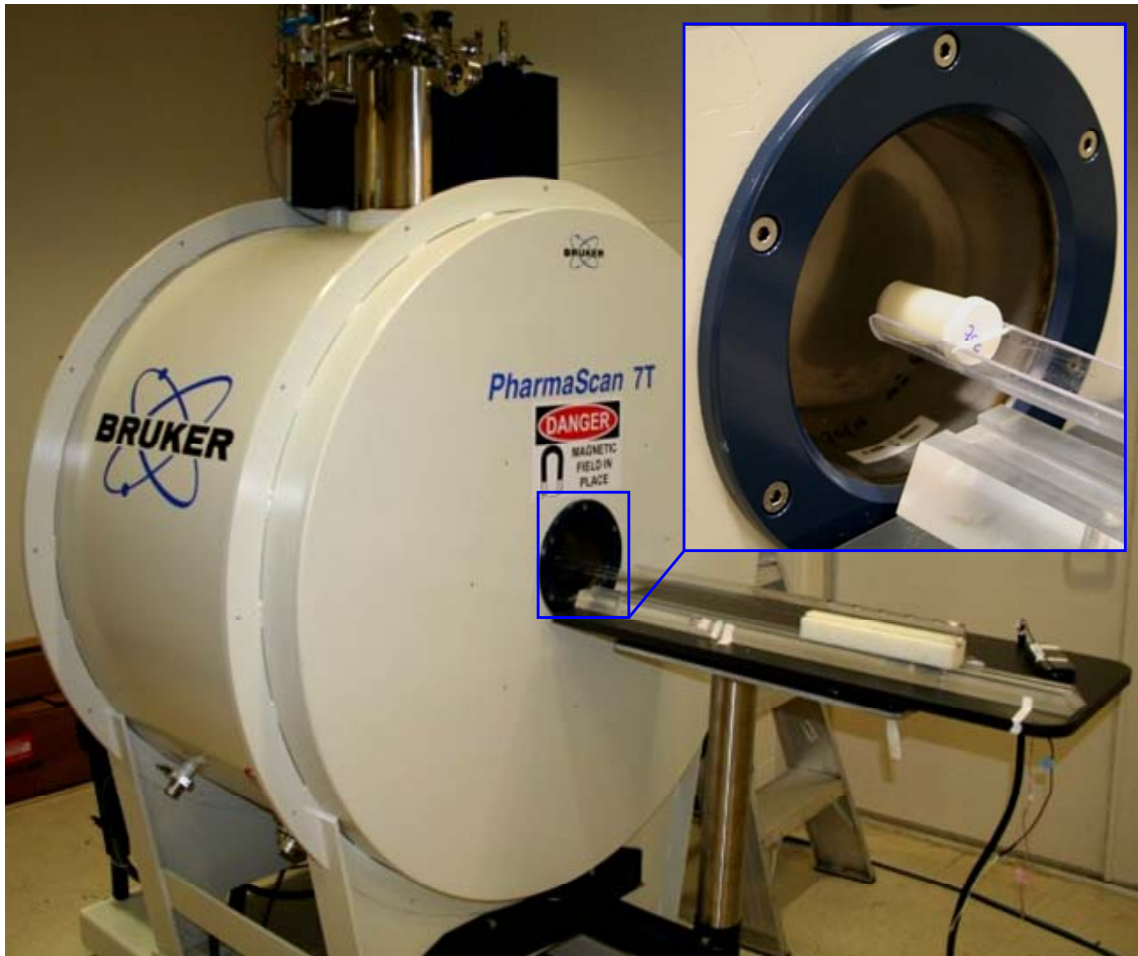
Figure 3.5: MRI setup used for scanning the gels.
