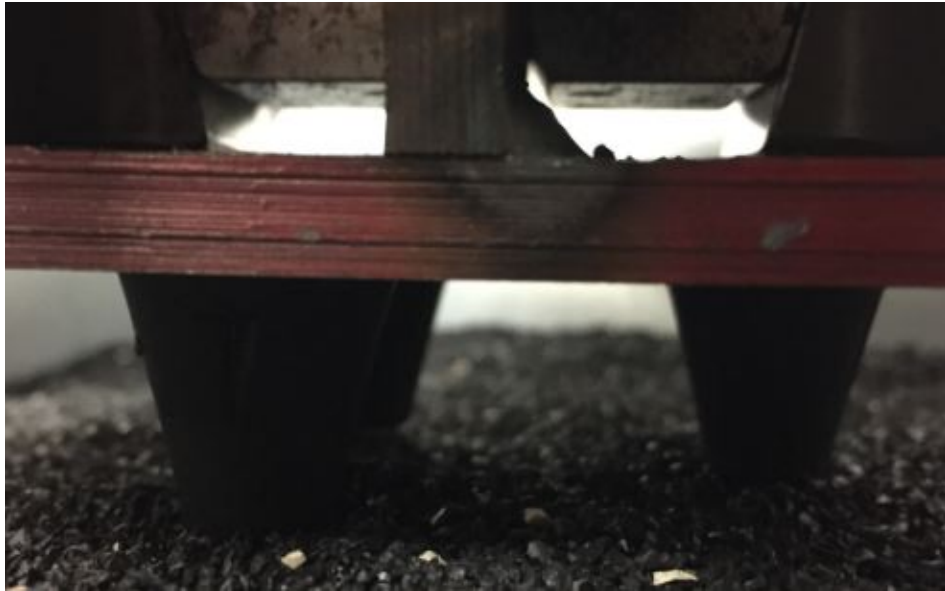
Figure 3.2: Showing Light Contact Between the Studs and Infill
