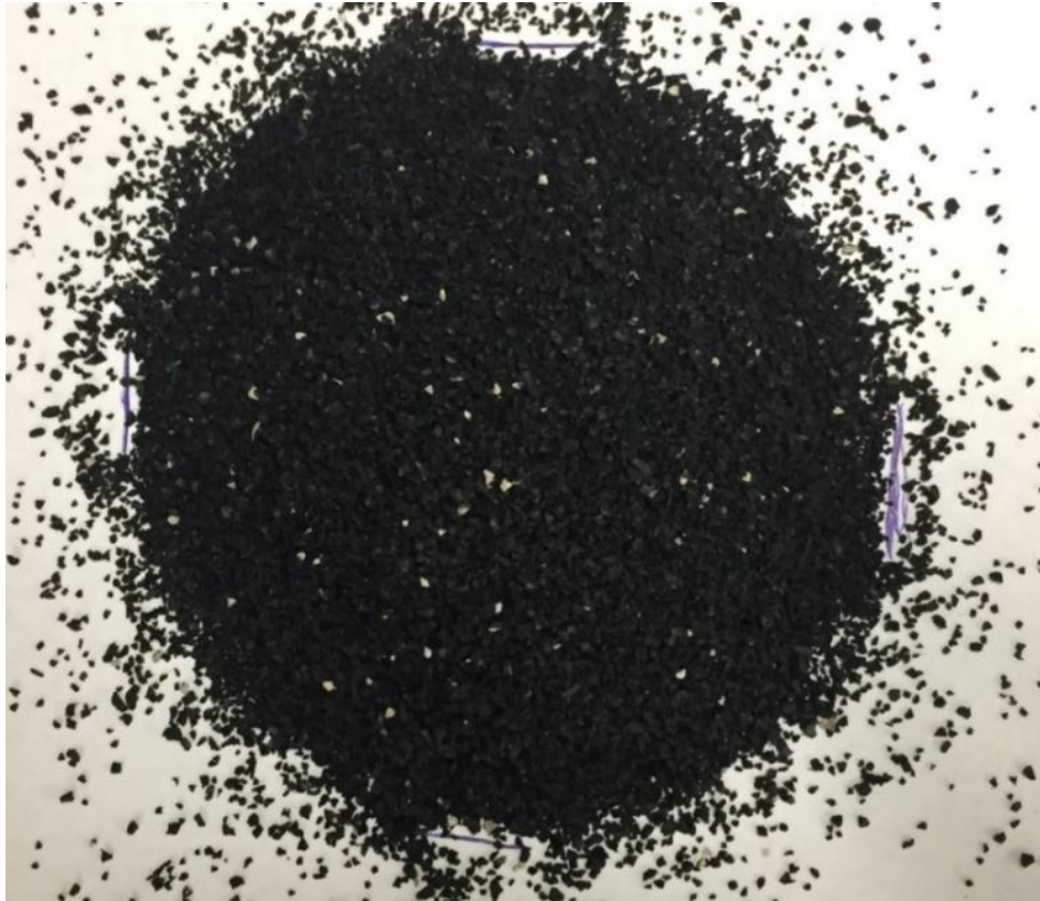
Figure 3.5: A Pile of Infill After an Angle of Repose Test
