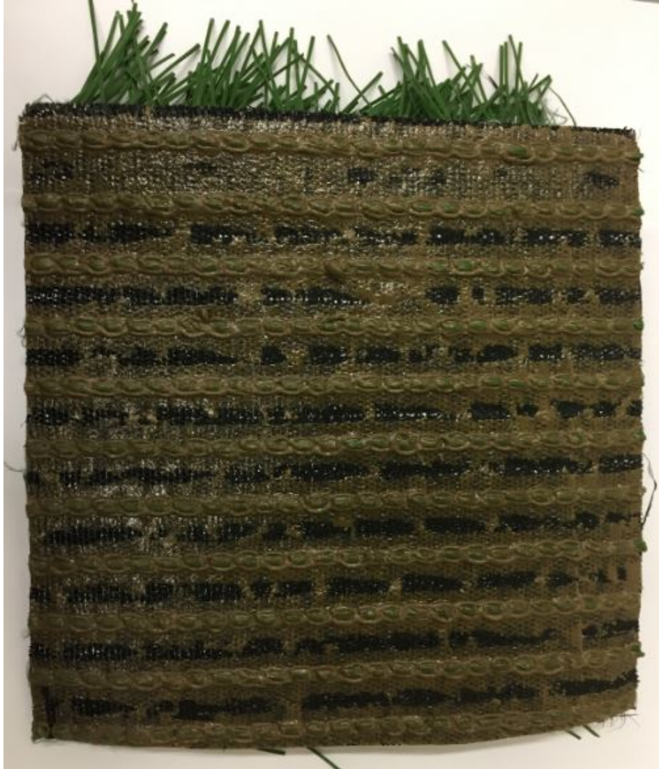
Figure 3.11: Backside of the Artificial Grass
