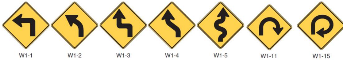
Figure 1 – Advanced curve warning signs for Horizontal Curves
