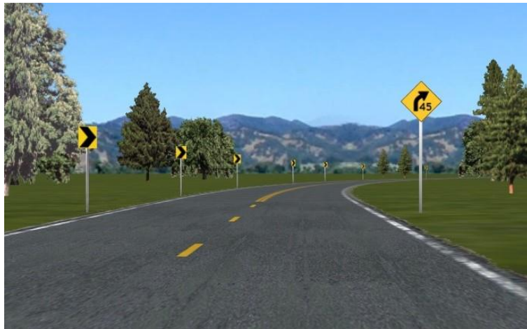
Figure 6 – Scenario showing Advance Curve warning and Chevron sign
