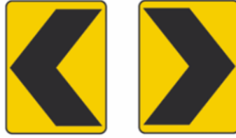
Figure 2 - Left and Right Curve Chevron sign
