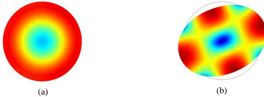
Figure 4.1 – Comparison of the finite-element simulated mode shapes for a 30 \mu\text{m} -diameter ZnO-on-silicon disk resonator with a 20 \mu\text{m} -thick device layer and a 500 nm-thick ZnO layer operating in its radial-contour mode at 88.43 MHz and wine-glass mode at 65.28 MHz
