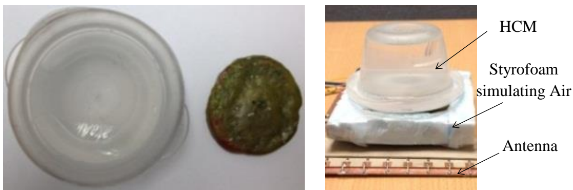
Figure 4.23: HCM consisting of a solid skin-muscle tissue phantom and liquid blood-fatty tissue phantom (left), antenna at 20 mm separation from the HCM (right).
