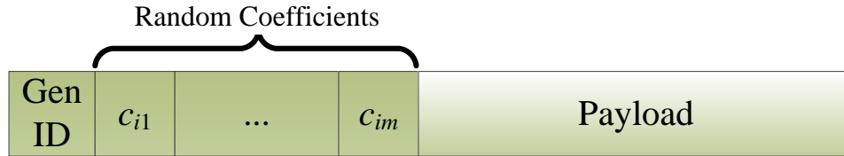
Figure 2.7 Network Coding packet format
