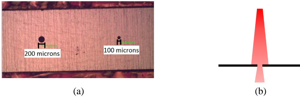
Figure 2.3: SEM column apertures. (a) Shows an actual adjustable aperture plate with four apertures. (b) Shows an illustration of an aperture acting on the primary beam.
