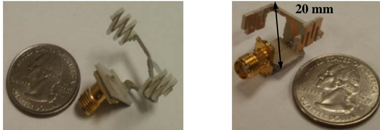
Figure 6.5: A photograph of the 3-D machined substrate cube antenna fabricated with the FDM process (left) and fabricated with the PCB technology (right).
