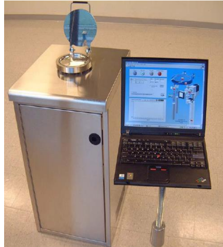
Figure 2.5 Savannah 100 ALD system by Cambridge Nanotech Inc. used in this work.
