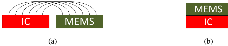
Figure 1.5 MEMS-IC integration by (a) hybrid approach and (b) monolithic approach [12].
