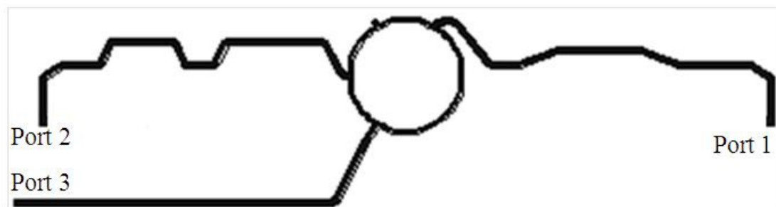
Figure 3.11 Rat-Race coupler used in each single-fed sub-array architecture.
