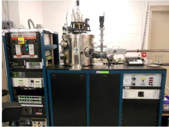
Figure 3-1: AJA RF Sputtering System
